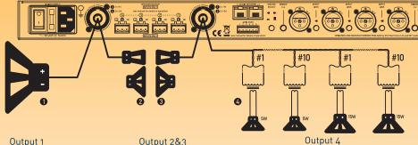
Output 1 Low Z sub (mono) Output 2&3 Low Z cabinets (stereo)
