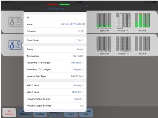
Once connected, all the amps appear on the default "All Devices" view, and real time metering should start.
