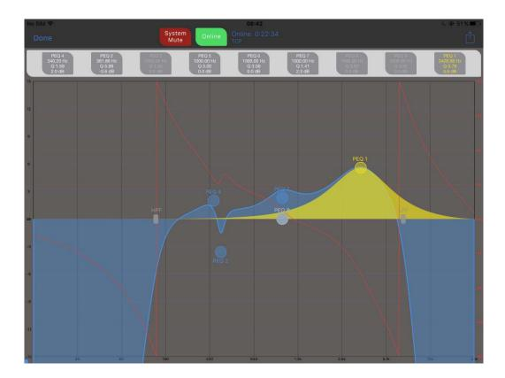
Drag filter nodes to adjust frequency and gain. Pinch to adjust filter 'Q'. Touch the filter information above the graph to edit directly with sliders and numeric input.
