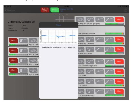
Still in the device view, grouping is shown beside channel names, and channels in an absolute group cannot have EQ directly editing here. Channels in relative groups (a channel can be in multiple relative groups) can still have their gain, delay and if an output, limiter threshold changed, and any additional offset is shown in brackets beside the readout.
