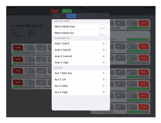
Touch routing matrix to access routing, channel ganging and channel naming. Full matrix mode can also be enabled independently for the power amplifier channels and aux channels.
