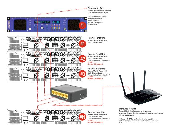
DeltaDirect connects to your WiFi network and to your DPA amplifiers via a wireless router. All amplifiers must be connected via their Ethernet control port to the router, and we recommend that there is a DHCP Server on the system to issue IP addresses automatically (this is normally the case and most routers have this feature built-in - Ethernet **switches** may not so check the specs!)
