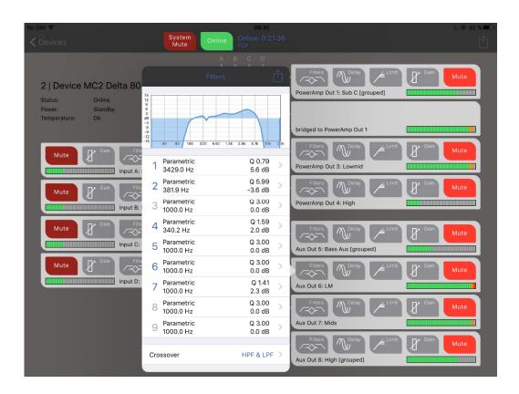
Individual bands may be edited by touching them in the table and directly moving slides or typing in values. On outputs, the crossover filters are accessed at the bottom of the table. Bypassed bands numbers are grey (like 3, 8 and 9 above). Touch the options top right on the window to reset all bands and access copy and paste.
