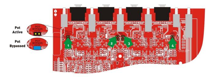
Adding a link to CN105 disables the pot for channel A, CN205 disables the pot for channel B, and so on.
