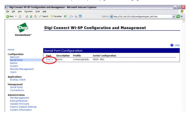
There is only one serial port on the WiSP, and as can be seen above, it's not yet been set up to our requirements, being both unassigned to any particular profile, and the actual serial settings being rather slow for AudioCore.
