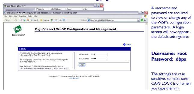
Below is the home page of the WiSP's device configuration. Note the IP address in the address window is the one that's just been set.
