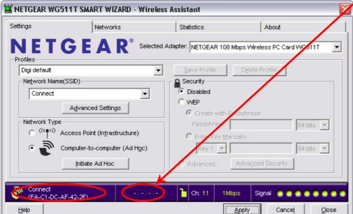
The Netgear card will now try to associate with the WiSP, the progress of which is indicated by the text in the blue pane turning red as the channels are cycled through.
