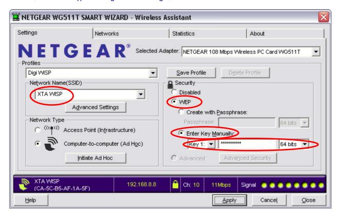
Set the Network Name to be "XTA WISP" - all capital letters, one space between the words (was previously set to "Connect"). Select WEP under the security settings (was previously set to "Disabled"), and enter the WEP key manually as "1234567890", and 64bit encryption.
