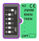
The standard "K2" converter has a set of DIP switches to adapt the system for various uses. These are set correctly by XTA when leaving the factory and should not be adjusted. If for any reason they are different, the correct settings are shown in the diagram to the left.
