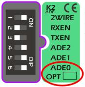
Check the DIP Switch label on your converter to see if it has been marked to show whether or not the following modification has been applied. If the "OPT" box is marked, then the converter is 115k capable. If not, then you will need to apply the modification.
