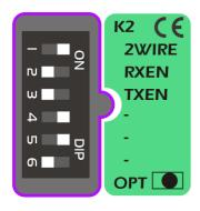
38400baud - Switches 1, 4, and 5 are ON.
