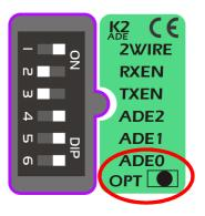
The switch settings shown above for the NON-modified version are correct for 38k400 operation. On the modified unit, this setting now represents 115k.
