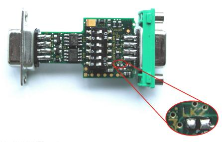
Locate the pair of solder pads labelled LK2.
