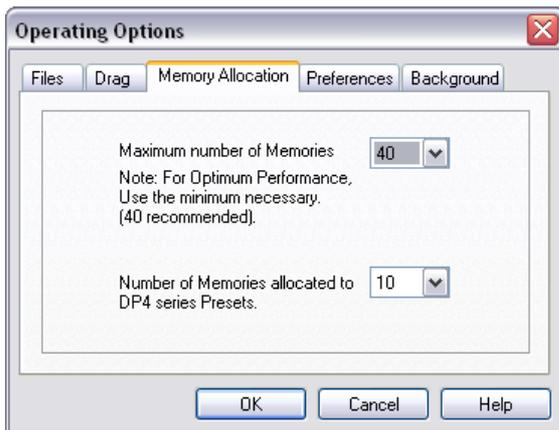
Choose the number of memories you require to upload to the PC. The number of presets doesn't matter in this case as whilst they can be imported into the software, they cannot be exported back to a unit as they reside in Flash and can only be loaded through a preset "bin" file dump.
