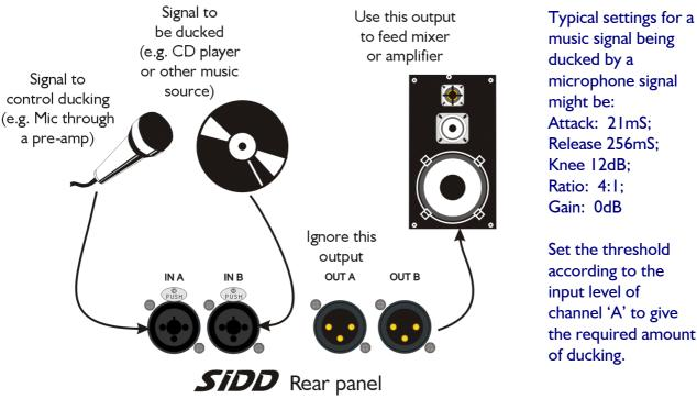
music signal being ducked by a microphone signal might be: Attack: 21mS: Release 256mS: Knee I2dB; Ratio: 4:1: Gain: 0dB
