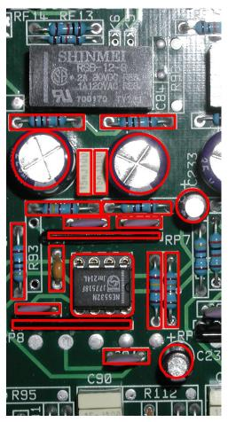
Note that the channel shown here is NOT channel I for a reason – there are two extra components near this channel that have to be removed to fit the transformers – they are the two smaller electrolytic capacitors circled on the right on the picture – C232 and C233 (47uF, 25v).
