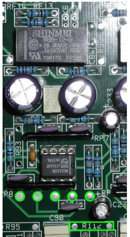
Once the big electrolytic caps have been removed (not removed on this pic) the other set of holes for the transformer will be visible. The first set is circled below in green. These holes will need to be cleared of solder.
