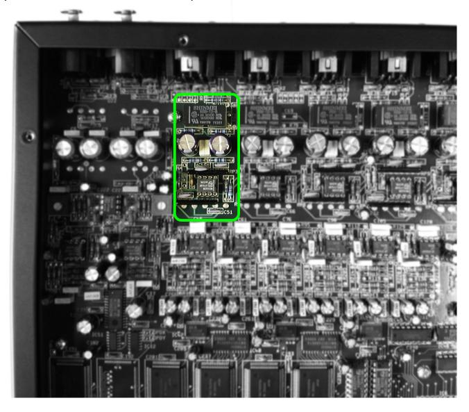
The picture below shows a close-up of this circuitry, and all components highlighted in RED must be removed. Hint – the majority of the components can be cut off the top of the board with a pair of side-cutters, but it is best to desolder the IC socket. Note that the transformer will be sitting over these old component locations and as such can potentially short against them so the removed components MUST be cropped very close to the board. If in doubt, desolder them.
